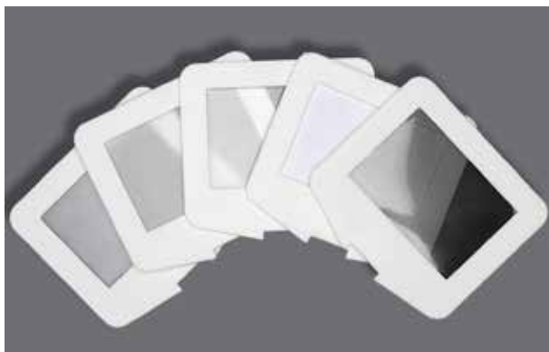
Fig 4 Five commonly used diffuser materials were chosen for the study. They included polyethylene (PET), White Frost photographic paper, LumiQuest polyamide (nylon) material, 80 gsm white printing paper, and 3M linear polarizing filter sheet used for cross polarization. Each frame had an open window of 80 mm x 55 mm.
