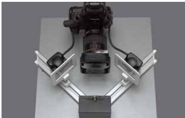
Figs 2 and 3 The experimental setup consisted of a DSLR camera paired with a twin flash commonly used for dental photography. In order to minimize specular reflection from the labial surface of the teeth, both electronic flash guns were arranged in two azimuthal illumination angles corresponding to 0 degrees/45 degrees geometry using two aluminum rails and two custom 3D-printed variable sled assemblies.
